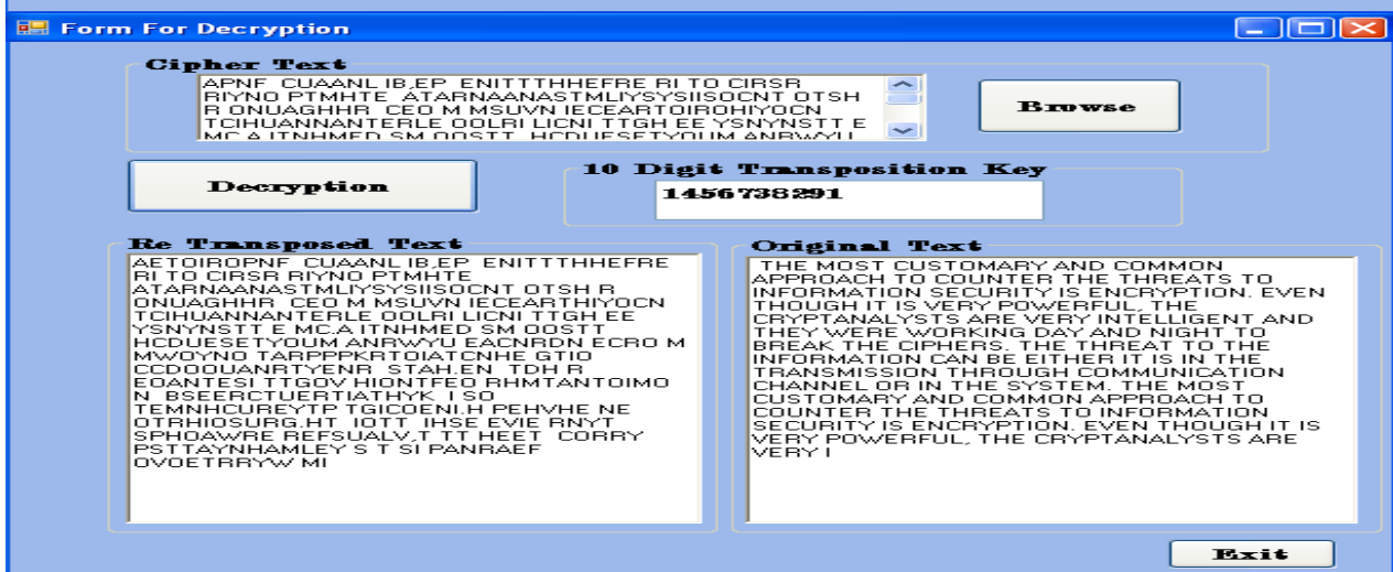
Figure: 3 A Screen Shot of Decryption Process using Tree Transposition Algorithm
