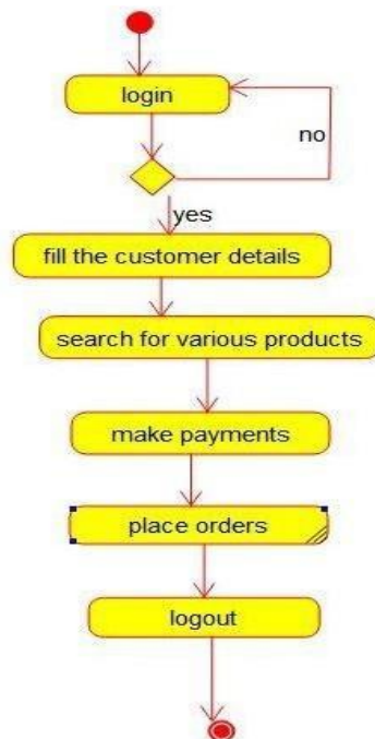
Figure 7 : Activity Diagram for Customer in Stock Maintenance System
